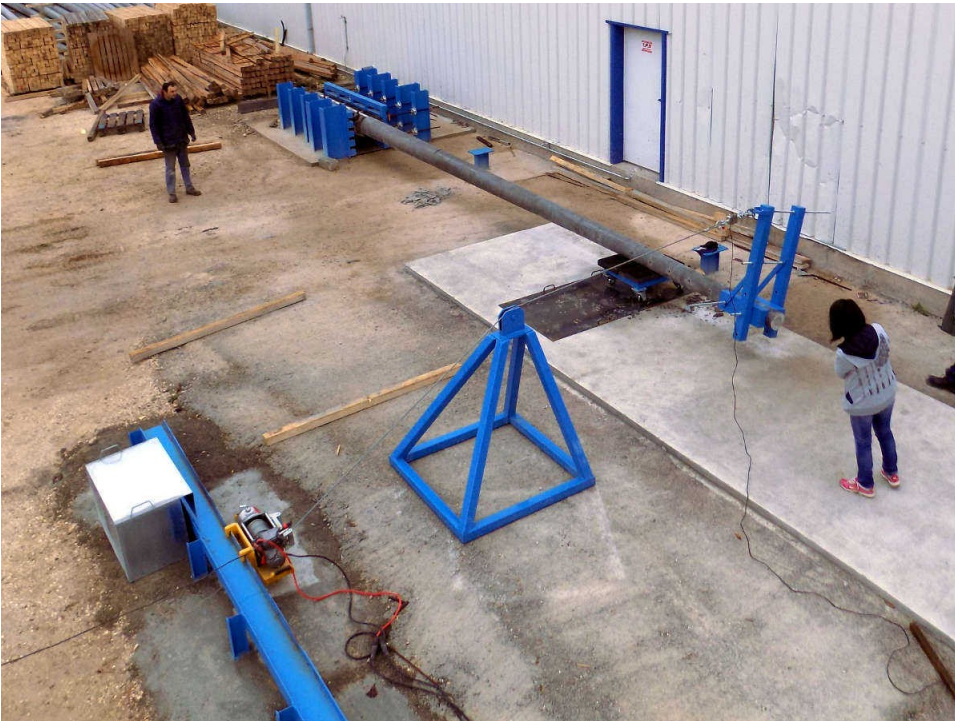
Pic. 5. Pole testing in combined bending and torsion
