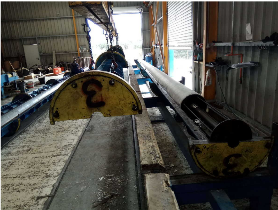
Pic 2. Mold on the demolding bench. The upper half is already removed
