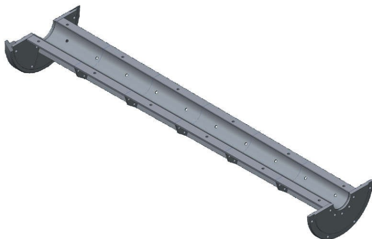
Fig. 1. Half 3-meter mold (interior)
